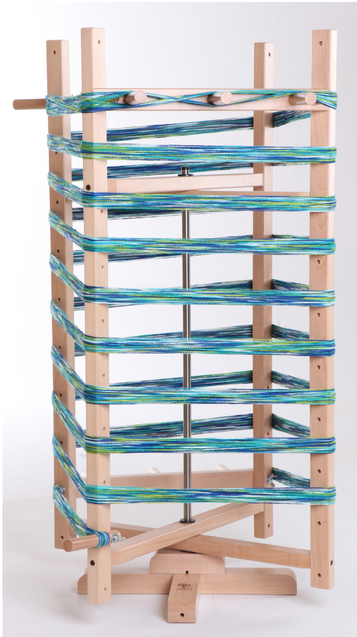
The threading cross - each thread is crossed.
