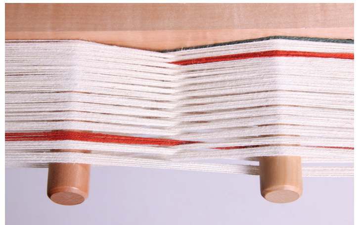
The raddle cross - threads in groups of 10 crossed.
